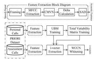
Figure 1: Schematic block diagram of i-vector extraction.
